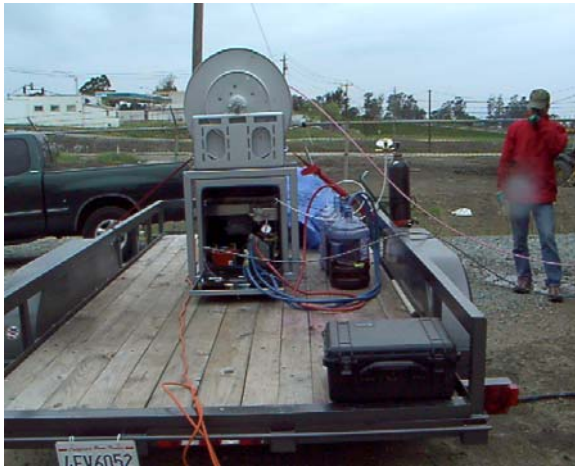
Figure 5: Electrical and Pneumatics components inside housing are controlled by the Dye Injection Control Unit (Figure 4). The housing contains injection pump, injection pressure regulator, pneumatically controlled valve switching solenoid, fuse box, electrical circuits and primary and secondary valve control units.
