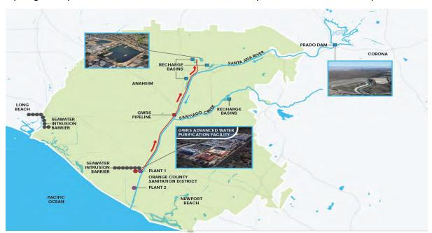
The system takes treated wastewater from the Orange County Sanitation District, water that would have otherwise been discharged to the ocean, where it undergoes an advanced water purification process to produce 130 million gallons of high-quality drinking water every day.
