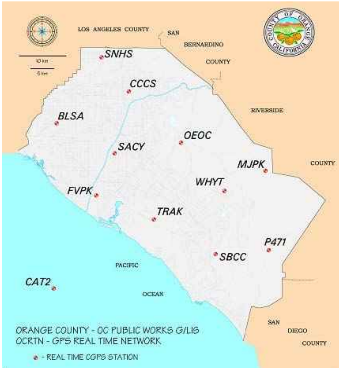
Figure 13-1: Orange County Public Works GPS Real Time Network
