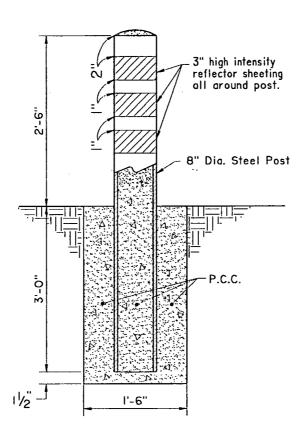
Required to protect signals or street lights adjacent to driveways (Minimum 2 ft. clearance).
