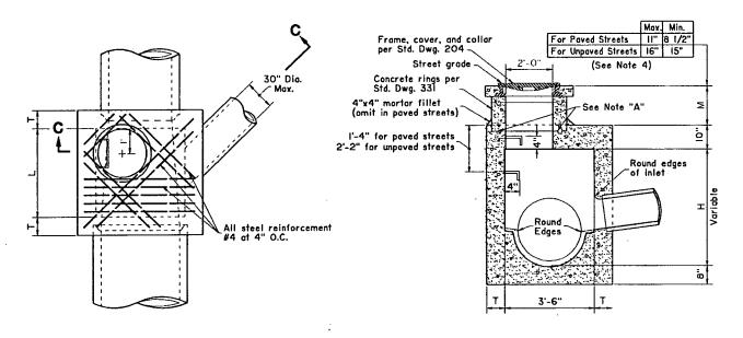
PLAN See Note 3 Note "A"-Two (2) inch deep seat to correspond to manhole shaft, grout between shaft and seal.
